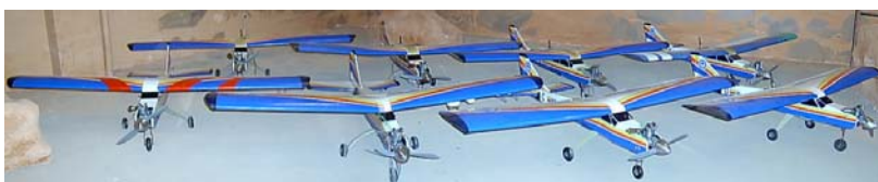
(a) Fleet of eight identical Trainer 60 aircraft used in the multi-UAV testbed at MIT.
