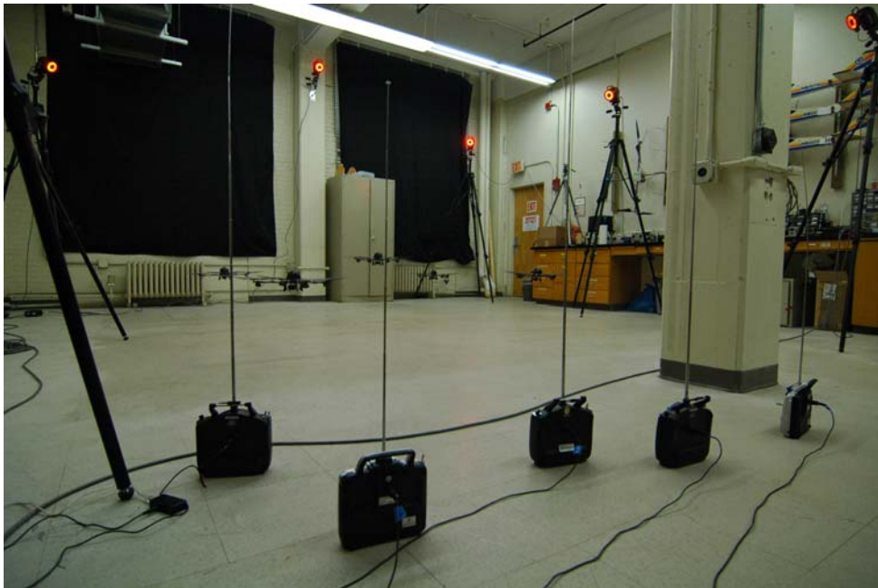
Figure 3: RAVEN infrastructure required to fly five autonomous quadrotors [20]. The bright LED rings show the location of the Vicon cameras. The Vicon data is processed in a central computer and then distributed to the ground flight computers that are dedicated to a particular vehicle. This position data is processed using the current mission plan (developed in a second set of distributed computers), and the signals are sent directly to the UAV's actuators using the RF transmitters.
